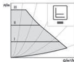
Recommended for underfloor heating or for large-sized pipes, applications without a variable pipe network curve (e.g. storage charge pumps) or single-pipe heating systems with radiators.
