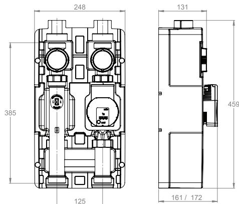
**LK 862 - PUMP GROUP WITH MIXING VALVE | PUMPENGRUPPE MIT MISCHVENTIL | GROUPE DE POMPES AVEC VANNE DE MÉLANGE | GRUPPO POMPA CON VALVOLA DI DERIVAZIONE | PUMPPURYHMÄ SEKOITUSVENTTIILILLÄ | PUMPGRUPP MED SHUNTVENTIL**
