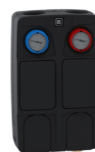
LK 867 - Pump group with a four way mixing valve, LK 830 ThermoMix® B. Without pump
