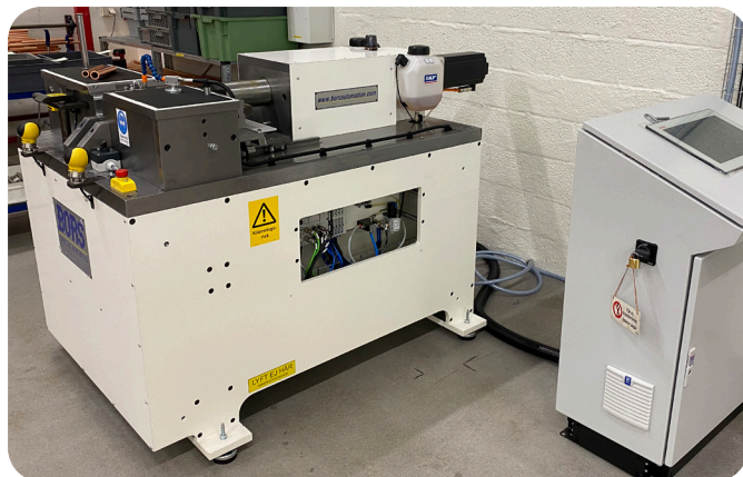
End forming machine on our production line.
